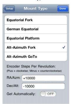
Under 'Encoder Steps Per revolution' set both 'RA/Azm' and 'Dec/Alt' to the number of steps per revolution of your corresponding encoders (10000 in this example). Please turn off 'Get Automatically'.
