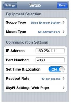
Under 'Communication Settings': set the 'IP address' to 169.254.1.1, 'Port Number' to 4060. Set 'Scope Type' to 'Basic Encoder System'.
