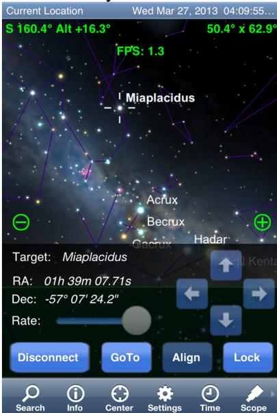
By pressing the 'GoTo' button ServoCAT will slew to the object:
