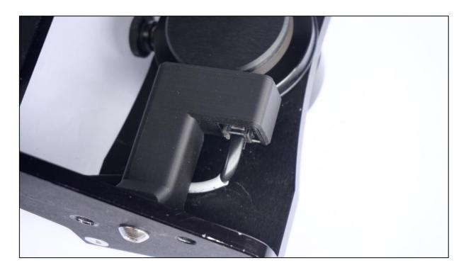
Now insert the altitude encoder lead plug into the altitude encoder readhead with contacts facing down:
