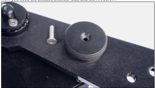
Put the encoder disk on the shaft and push it all the way down:
