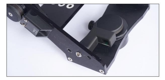
Now you need to check the gap between the readhead and the magnetic ring's surface. As in case of the altitude encoder the gap should not exceed 0.8mm:
