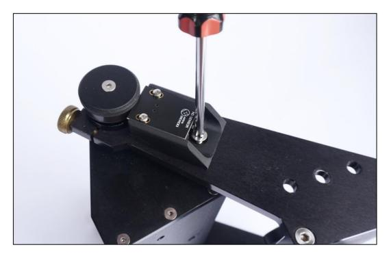
**NOTE:** You need to check the gap between the encoder ring and the readhead. The gap should not exceed 0.8mm – it can be as small as possible without the readhead touching the surface of the ring:
