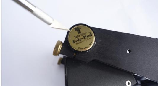
Then you need to remove two screws using the 5/64" hex key:
