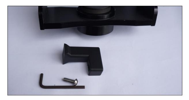
Position the readhead aligning the mounting hole with the centre hole of the right arm and put the screw through the hole:
