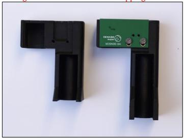
Now you need the azimuth encoder readhead, ¼" button head screw and the 5/32" hex key:
