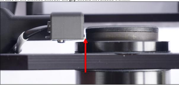
In case it needs to be adjusted you need to remove the readhead, loosen the screws holding the green PCB and move the PCB forward/backward to adjust the gap. Now feed the azimuth encoder cable lead under the readhead and insert the plug into the readhead with contacts facing up:
