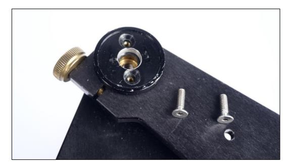
Next put the altitude encoder disk shaft on top aligning holes with the holes below and threaded holes:
