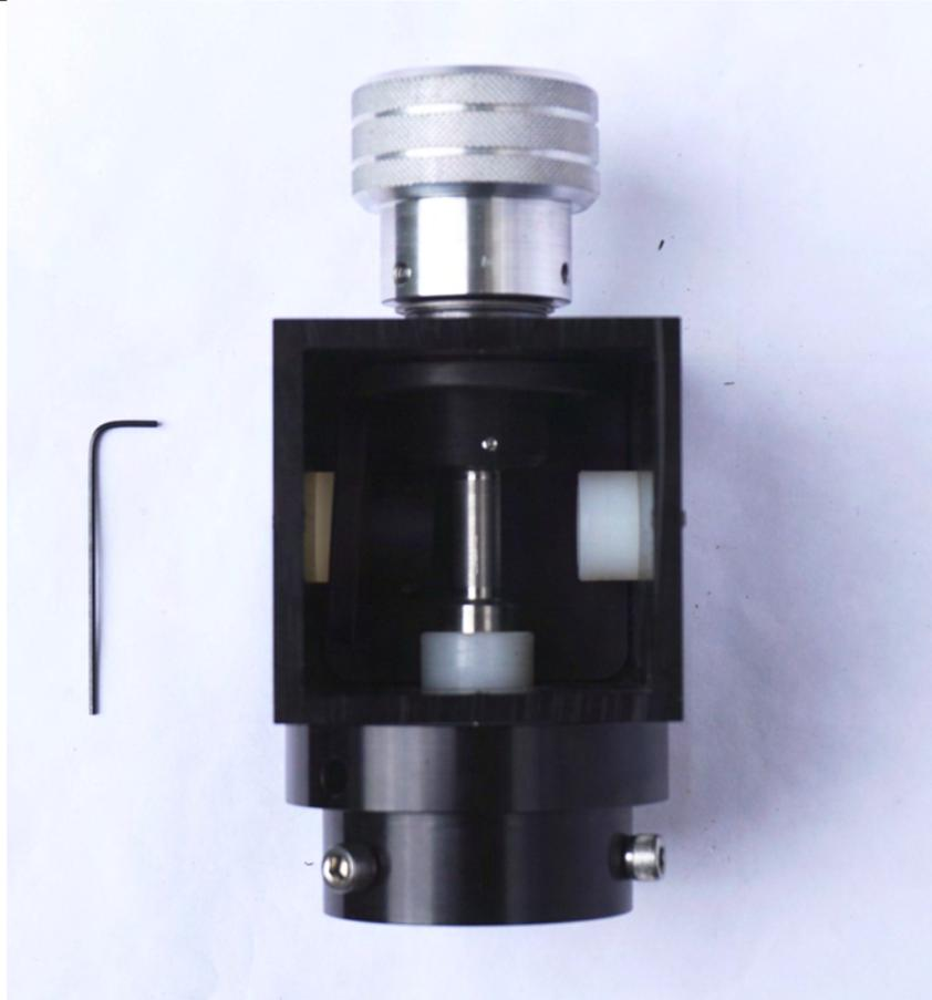
Now tighten the set screws on the encoder disk using 1.5mm Allen key (5) – just lightly (the encoder disks have a very tight fit). You may need to loosen the adjustment knob to be able to rotate the shaft to gain access to other set screws.
