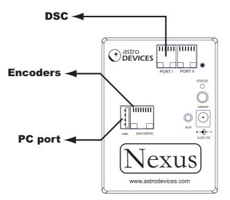
Where 'DSC' and 'PC Port' are the names of the ports on ServoCAT. Please note that a two star alignment should be performed before ServoCAT can track and execute goto commands.
