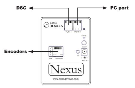
Where 'DSC' and 'PC Port' are the names of the ports on ServoCAT. Please note that a two star alignment should be performed before ServoCAT can track and execute goto commands.
