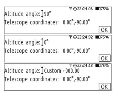
The custom angle can be set with a precision of 1/100 of a degree. Once *Custom* is selected you can change the integer part (from -180° to +180°) using and keys:
