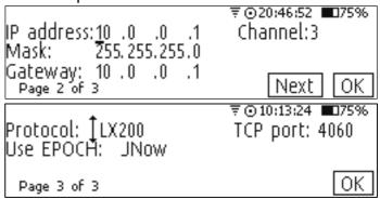
The **Use EPOCH** is set to **JNow** by default as most planetarium applications use the current epoch for the coordinates. Some planetarium applications can only accept **J2000**.
