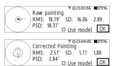
If you the results are suitable then you can enable using the calculated model for telescope pointing:
