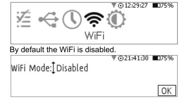
The easiest way of using Nexus DSC with a smartphone/tablet/laptop is to switch the WiFi to *Access Point* mode:
