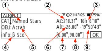
Nexus DSC shows the current azimuth and altitude for the selected alignment object (2) and 6 above)
