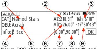
Nexus DSC shows the current azimuth and altitude for the selected alignment object ((2) and (6) above)
