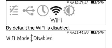
The easiest way of using Nexus DSC with a smartphone/tablet/laptop is to switch the WiFi to *Access Point* mode:
