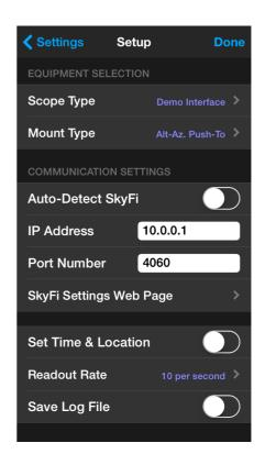
Nexus DSC is emulating LX200 protocol when used with a planetarium application. Change the **Scope Type** to **Meade LX200 Classic**:
