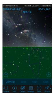
Now SkySafari Plus/Pro should show a telescope cursor on the screen. Moving the telescope will result in the cursor movements on the screen. If the Telescope cursor moves in the opposite direction in either of the axis then you need to touch 'Disconnect', go to SkySafari's Settings->Telescope-Setup and change the sign in front of the encoder steps to opposite (from '+' to '-', for example) for the corresponding encoder(s).
