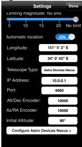
Set the 'IP address' to 10.0.0.1, 'Port' to 4060. Set 'Alt/Dec Encoder' to the number of steps per revolution of the altitude/declination encoder (10000 in this case). Set 'Az/RA Encoder' to the number of steps per revolution of the azimuth/right ascension encoder (10000 in this case). Set 'Initial Altitude' to either 90 degrees or 0 degrees. It is also advisable to set 'Automatic Location' to 'ON'. Touch 'Done'.
