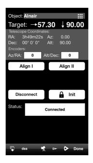
7. Now point the telescope at the selected star (Alnair in this case) and touch 'Align I'. A tick mark will appear on the button. Now select a second alignment star (Alshain in this case), point the telescope at the star and touch 'Align II'. A tick mark will appear on the 'Align II' button. The alignment error will be reported in the status window (0.10 here) – the smaller error the better pointing accuracy will be achieved.
