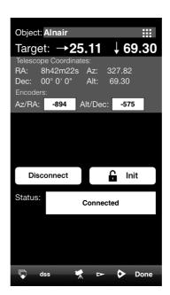
**Note:** Please make sure that Az coordinate is increasing when rotating the telescope clockwise and Alt coordinate is increasing when the telescope is moved up. Change the sign for the corresponding encoder steps to opposite in the settings if the coordinate is changing incorrectly.
