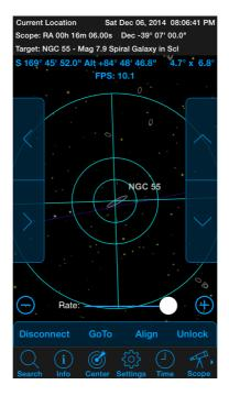
You can now select an object in SkySafari and touch the GoTo button on the telescope control panel and the telescope will slew to the selected object.
