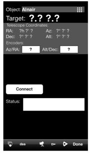
**5.** Touch 'Connect'. The screen will now show the current encoders' position and coordinates. The coordinates will only be valid once the two star alignment is performed.
