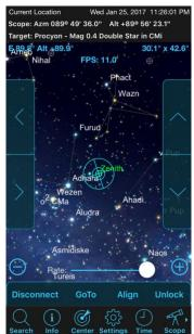
Now select a star and point the telescope at the selected star. *Betelgeuse* was selected in this example. The telescope cursor will most likely be quite far from the selected star unless the telescope is levelled and pointing north when the altitude reference was performed. The telescope cursor does not have to be over the selected star:
