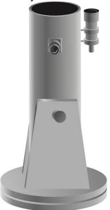
The same rule applies to telescopes installed on equatorial platforms. Please note that the telescope should be at 90 degrees to the ground board, not the ground.
