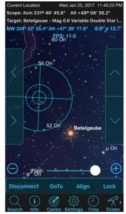
Once the star is precisely in the centre of the field of view touch the *Align* button. A popup window will appear to confirm the alignment:
