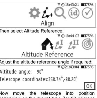
Now move the telescope into position depending on the mount type (for 90 degrees reference):
