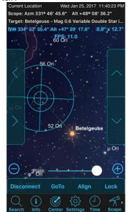
Once the star is precisely in the centre of the field of view touch the Align button. A popup window will appear to confirm the alignment:
