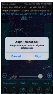
Touch the Align button to confirm. Nexus DSC will produce a short beep if sounds are enabled. The telescope cursor will now be located precisely over the selected star:
