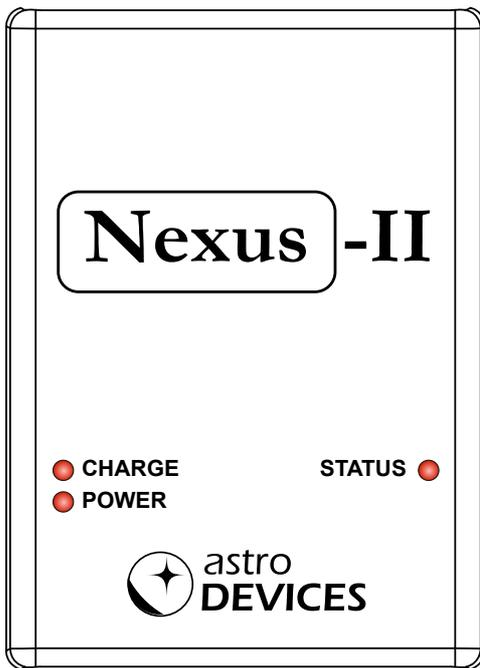
**CHARGE** – indicates if charging is in progress (ON if charging, OFF if charging is complete)
