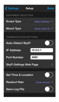
Nexus DSC *Pro* is emulating LX200 protocol when used with a planetarium application. Change the **Scope Type** to **Meade LX200 Classic**:
