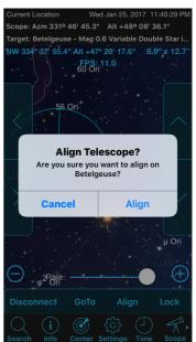
Touch the *Align* button to confirm. Nexus DSC *Pro* will produce a short beep if sounds are enabled. The telescope cursor will now be located precisely over the selected star:
