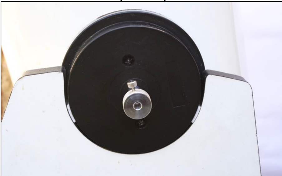
Insert the altitude encoder into the shaft adapter:
