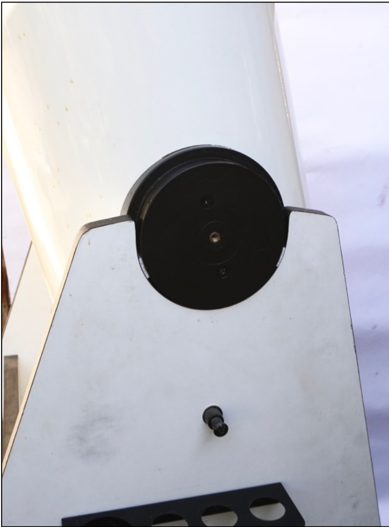
Screw the encoder shaft adapter in its place:
