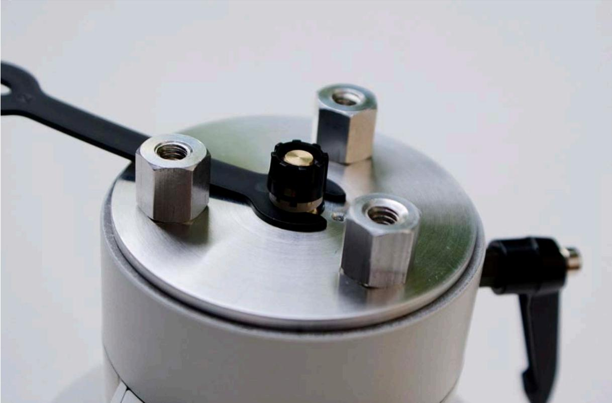
For the next step you will need the encoder base plate with a centering tool, two M2.5 screws and a screwdriver:
