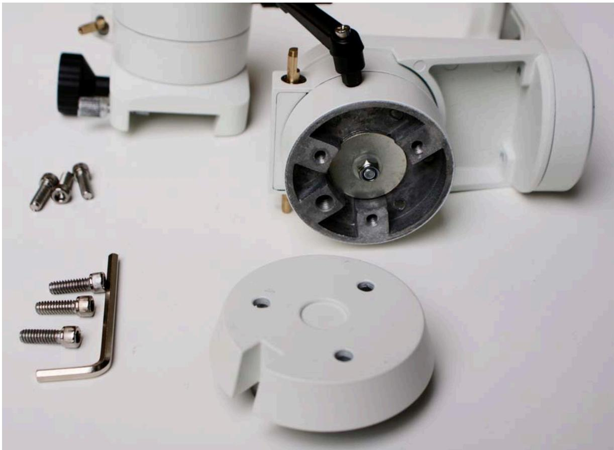
Remove the locking nut and leave the plastic washer on the axel:
