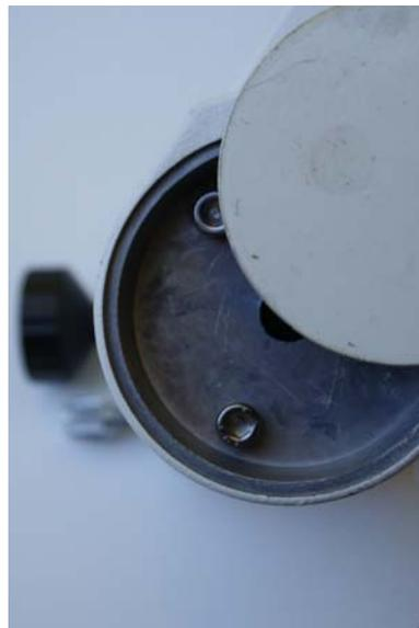
Remove the screws using the allen key supplied with the mount:
