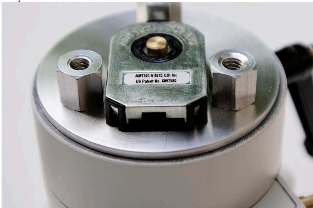
Plug the connector into the encoder:
