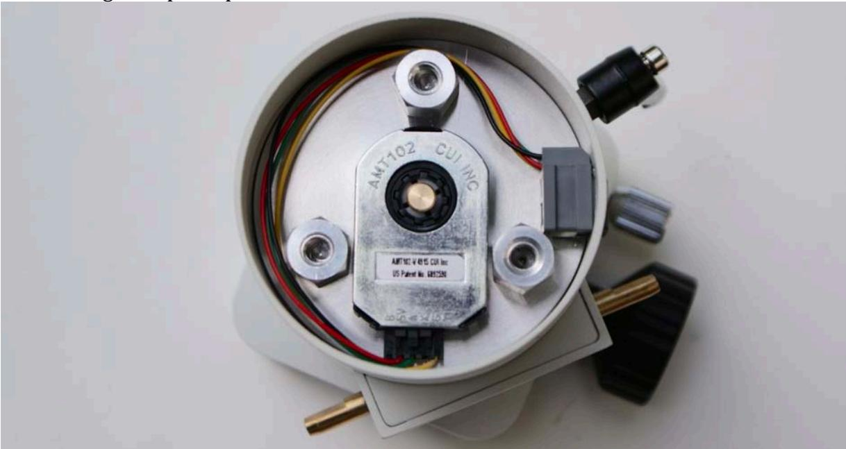
Place the assembled altitude encoder under the mount arm, put the screws back in and tighten them:
