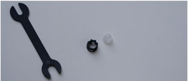
Place the spacing spanner over the encoder shaft and put the white shaft sleeve over the shaft:
