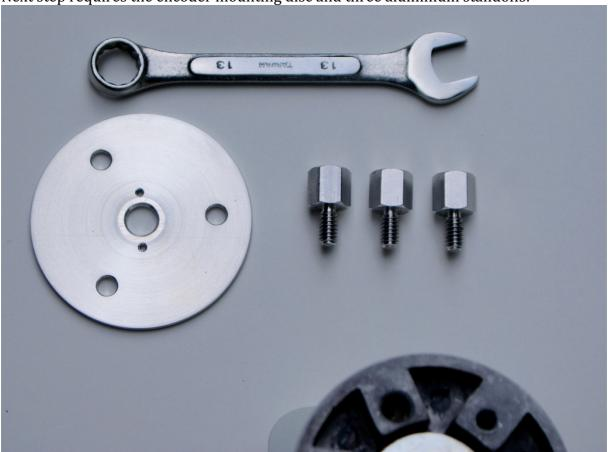
Place the disc on top of the mounting holes matching three holes on the disc to the threaded holes:
