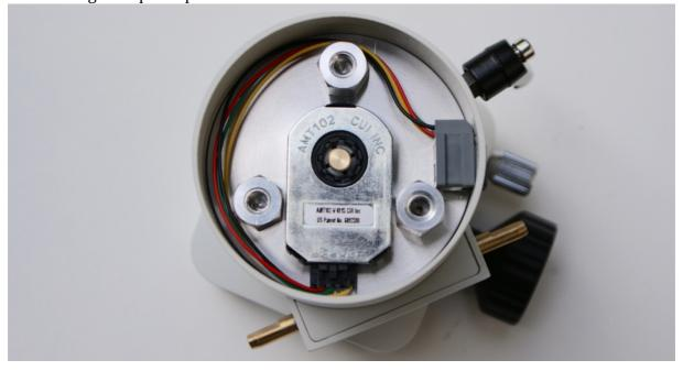
Place the assembled altitude encoder under the mount arm, put the screws back in and
