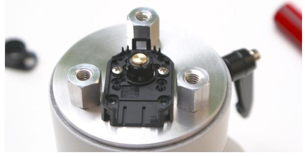
Place the centering tool on top – push it in. You may need to rotate the bottom part until the holes in the centering tool are over the screws:
