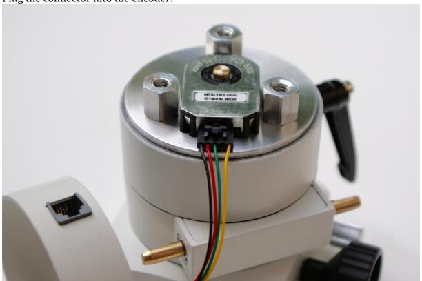
Put the ring on top and put the cable around the standoffs:
