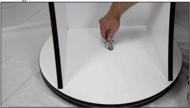
Tighten two set/grub screws using supplied Allen key
