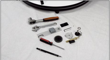
The azimuth pivot bolt needs to be replaced with the supplied azimuth pivot bolt. Use the socket wrench and the shifter tool/adjustable spanner to remove the pivot bolt. You also need to remove the existing plastic bushing from the hole.
