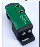
Slide the encoder reader over the left (front) bearing
