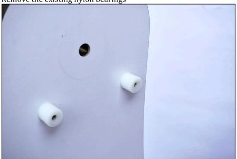
And install two bearings provided with the kit:
