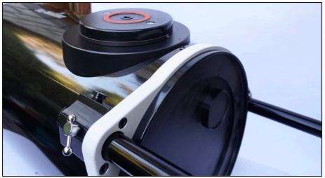
Now put the OTA back on the rocker box and make sure that the top of the reader PCB is a line tangent to the circle of the altitude bearing:
