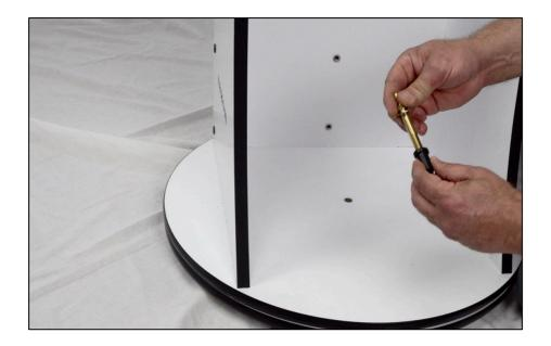
Put the rocker box on its side and install the aluminium plate on the pivot bolt. Drill holes for the screws using the supplied drill bit.
