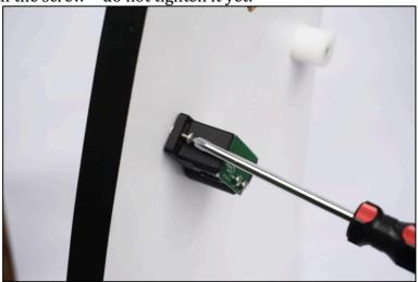
Put the OTA back into the rocker box and make sure the gap between the reader and the tape is  $\sim$ 0.8mm. Then tighten the screw:
