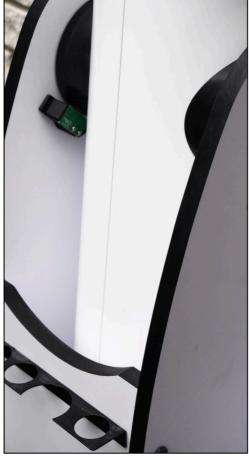
Now mark the altitude bearing just past the body of the encoder reader with a pencil (it might be easier to use something like a safety pin to put a small scratch instead):
