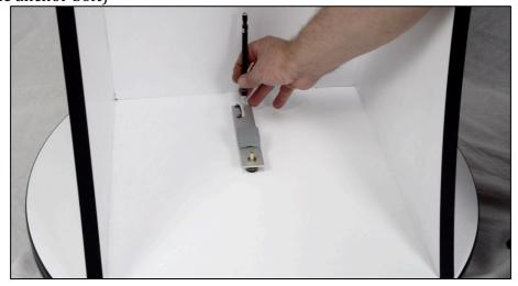
Swing the tangent arm away from the marked spot and put the anchor bolt with the foot on the marked spot. Then use the pencil to mark one of the holes
