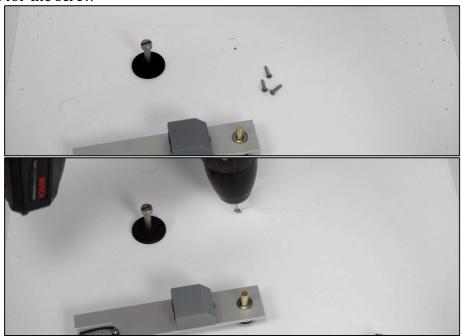
Fix plastic foot to the rocker box with three screws provided
