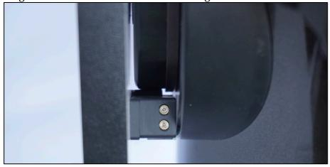
Remove the OTA again and use the pencil to mark the middle of the slot in the reader's housing:
