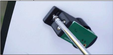
Put the OTA back on the rocker box and examine the gap between the encoder reader's top and the magnetic tape – it should not exceed 0.8mm (ideally it should be 0.4mm)
