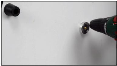
Use the supplied screws to secure the plate.
