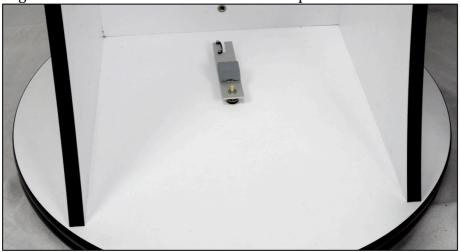
Use a pencil to mark the middle of the slot at the end of the tangent arm on the rocker box (for the placement of the anchor bolt)
