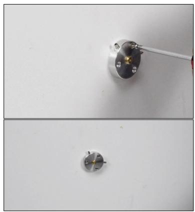
Tighten the pivot bolt making sure the rocker box still rotates as usual.
