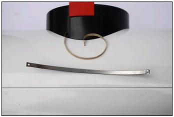
Use the spacing tool to control the distance of the tape from the edge of the bearing. Here the lower part of the OTA is on the left. Position the end of the magnetic tape starting from the marked position.
