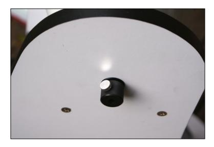
• Insert the Altitude encoder into the coupler:
