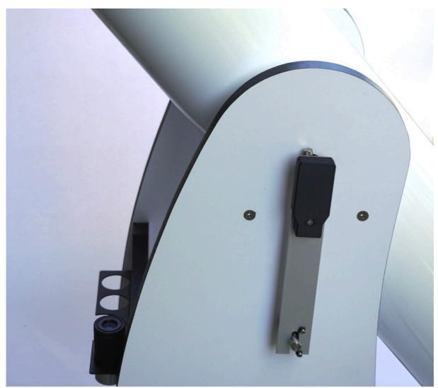
• Remove the encoder and fix the anchor bolt's foot with screws provided:
