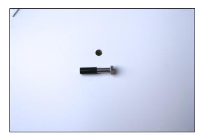
• Insert the bolt with the bushing into the hole in the ground board:
