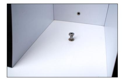
• Put the rocker box with the ground board on its side and fix the pivot bolt by tightening the set screw using the allen key provided:
