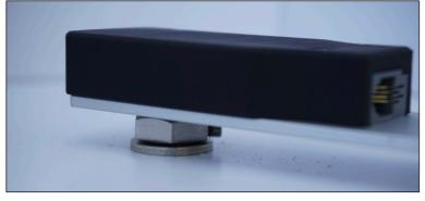
• Insert the anchor bolt into the slot on the encoder's arm, mark its place with a pencil:
