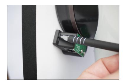
Drill a small hole for the screw:
