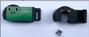
Put the screws into the housing and tighten them carefully (finger tight):
