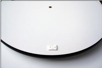
• Locate the new azimuth pivot bolt, insert it into the plastic bushing:
