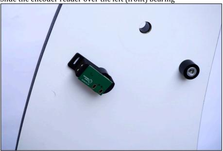
Put the OTA on the right bearing with the left bearing facing up. This bearing will be on the same side as the encoder reader when the OTA is installed on the rocker box.
