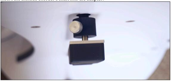
Then position the tangent arm at an angle (to the right or to the left but it should not be positioned vertically) insert the anchor bolt into the slot:
