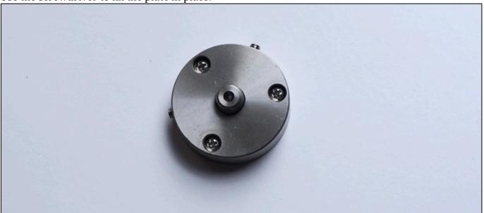
Tighten two set screws using the supplied Allen key (make sure that the rocker box can still rotate freely before tightening the set screws):
