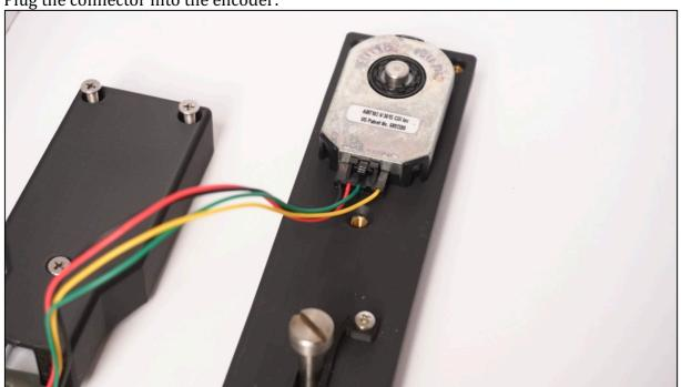
Put the housing onto the encoder and fix it with the supplied screws:
