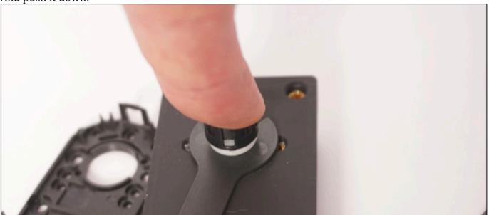
Put the encoder base plate and start threading the screws but do not tighten them yet:
