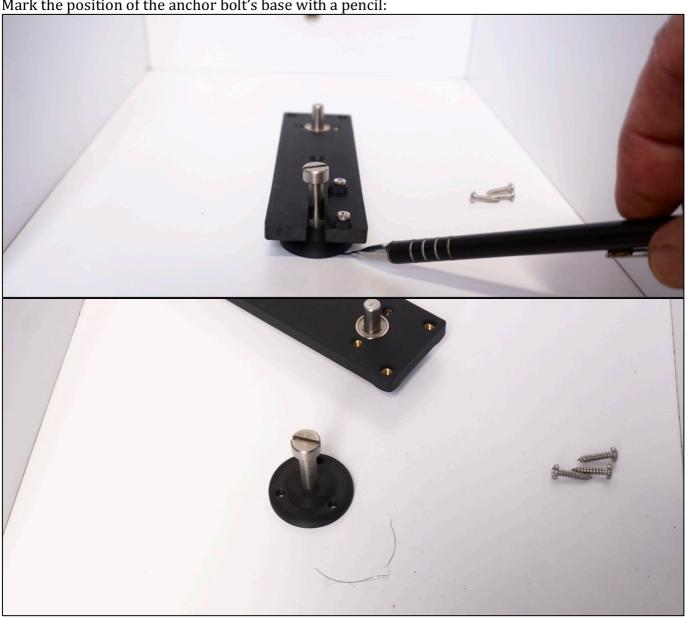
Unscrew the anchor bolt from its base. Drill holes for screws. Use the supplied screws to install the base of the anchor bolt:
