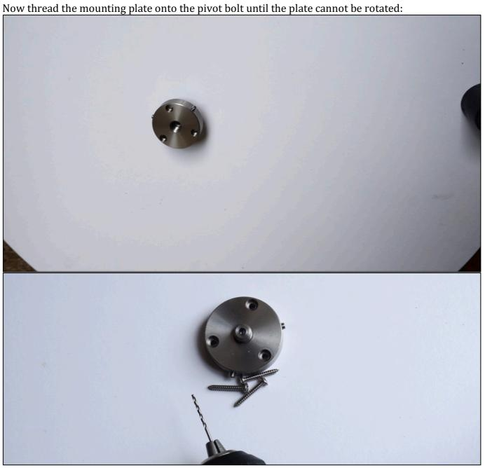
Now you need to drill a small hole using a 1.5-2mm drill bit:
