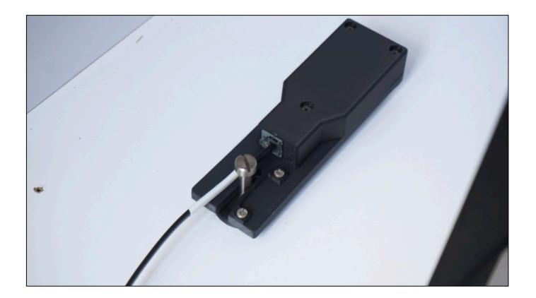
Please set the azimuth encoder steps to 8192 and altitude encoder steps to 8192 and follow the instructions of your DSC on setting the signs for the encoder steps correctly.
