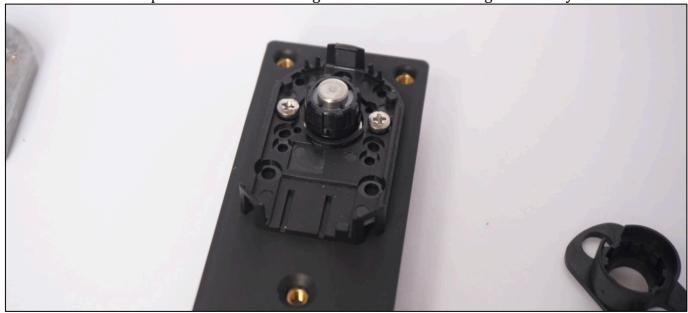
Use the alignment tool to centre the encode base plate:
