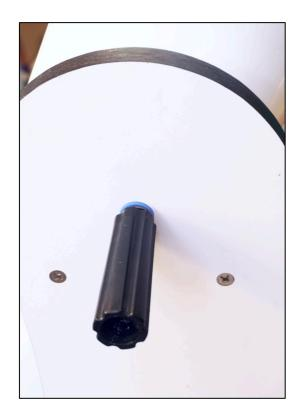
And replace it with the altitude encoder shaft adapter:
