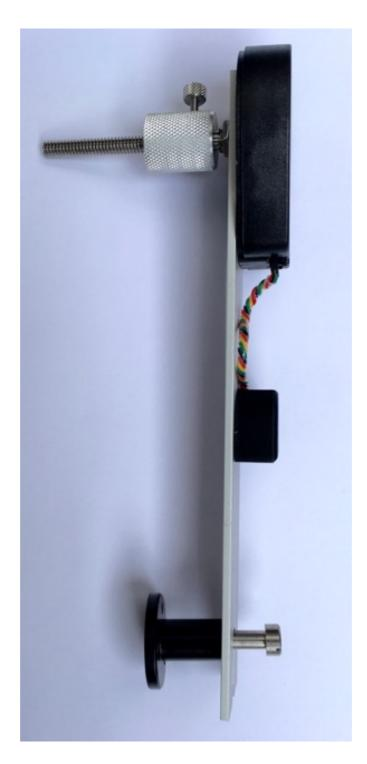
Connect the encoder cable and connect it to the DSC. Please set the encoder steps to 10000.
