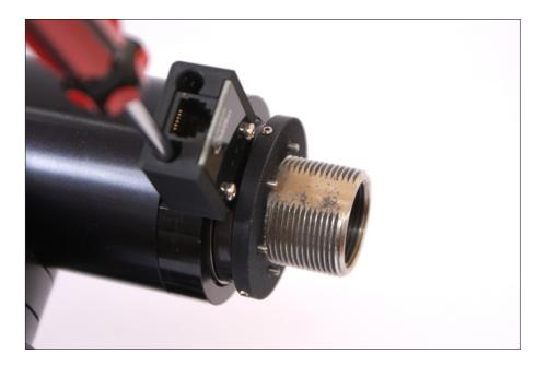
7. Tighten three set screws located on the encoder disk at  $120^{\circ}$  apart
