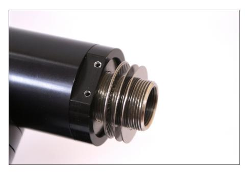
5. Then slide the encoder disk onto the shaft with the magnetic ring facing the washers:
