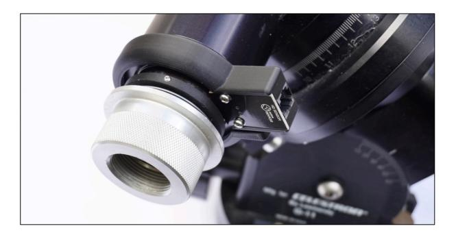
8. Tighten the encoder reader's clamp – please do not tighten it too much to avoid damaging the thread:
