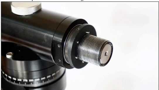
7. Then slide a washer, thrust bearing and another washer onto the shaft:
