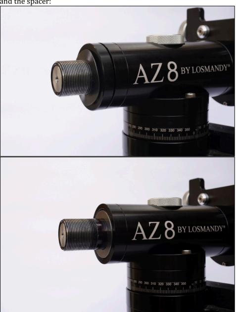
3. Install the encoder reader clamp – slide it over the end and push it all the way in:
