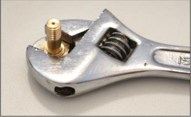
Now turn the base on its side and lock the pivot bolt with the lock nut:
