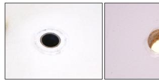
Then insert the bushing provided and push it into the hole:
