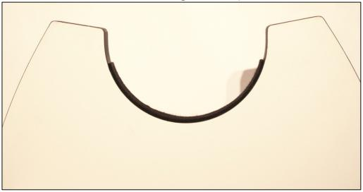
You will need to use the supplied template to mark the placement of the altitude encoder sensor. It is best to use a flashlight or another light source to place the template precisely on the inside of the side wall:
