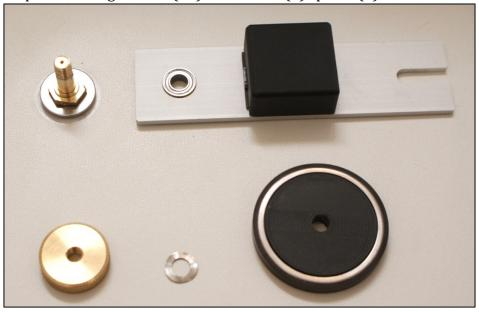
Feed the pivot bolt through tangent arm's ball bearing:
