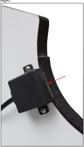
Put the OTA onto the rocker box and check the gap between the actual sensor and the magnetic tape. Adjust the placement of the sensor until the gap is 0.5mm or less and tighten the screws:
