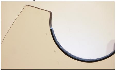
Now the magnetic tape (13) of the altitude encoder needs to be installed. You will need Isopropyl alcohol or similar solvent to clean the surface of the altitude bearing:
