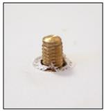
Now thread the plate onto the pivot bolt until the plate cannot be rotated:
