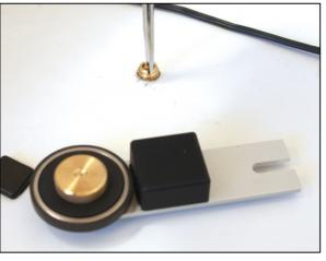
Move the tangent arm until the slot is over the threaded insert and thread the anchor bolt in:
