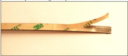
Remove the OTA from the rocker box. The magnetic tape needs to be glued very carefully on the inside of the altitude bearing starting from the line you marked in the previous step. For best results the ends of the tape should be glued with an epoxy glue (the adhesive needs to be scraped off in that case). Here only the adhesive of the magnetic tape is used. Use a soft cloth to put pressure on the tape while it is glued in place making sure it is fully adhered to the surface of the bearing:
