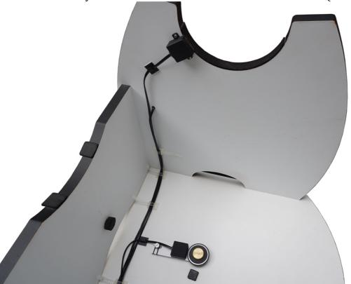
Note: the photo above shows the base of LightBridge 12" Deluxe with installed encoders and some additional wiring for dew heaters; the tangent arm shown is of previous revision without tensioning spring.
