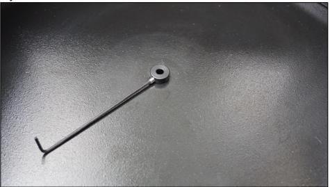
Clean the surface in the back with an alcohol wipe – where the encoder's foot will be glued. Remove the protective film from the encoder's foot:
