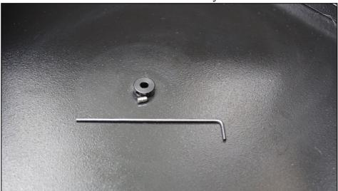
Put the set screw into the threaded hole and make a couple of turns but leave the Allen key in the set screw:
