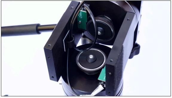
Install the side cover plate and then the top cover plate and connect the cable to your DSC.
