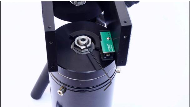
Insert the encoder disk and tighten the set screw:
